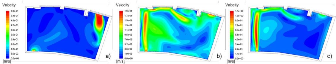
**Figure 4.** Maps of the velocity fields computed along the horizontal plane at 1.5 m above the floor in unsteady conditions (case UNST-A) at (a) 900 s, (b) 5400 s and (c) 7200 s.
