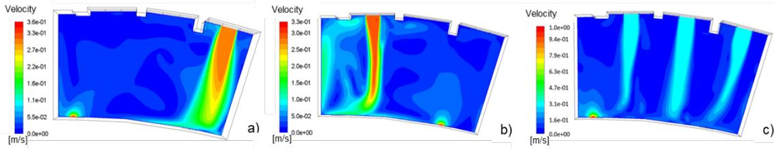
**Figure 3.** Maps of the velocity fields computed along the horizontal plane at 1.5 m above the floor for configurations A-B-C (Steady conditions).
