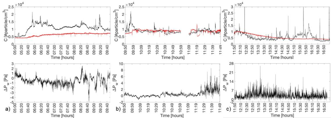
**Figure 2.** Indoor (red lines) and outdoor (black lines) particle concentration (top panels) measured at the window for different time intervals (interval-1 in panel a), interval-2 in panel b), interval-3 in panel c)) for IOP#1.
