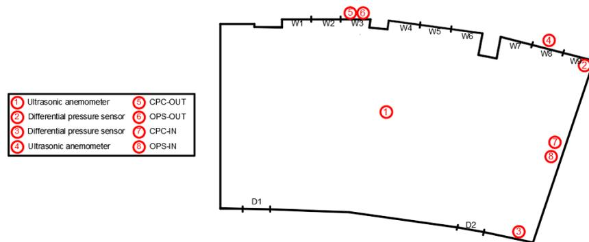
**Figure 1.** Layout of the classroom. The numbers indicate instrument positions during the IOP campaigns. D1 and D2 indicate room doors while the windows are denoted as W1-W9.
