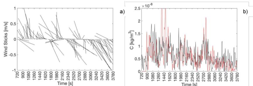
**Figure 5.** Stick plot of the external wind (a) and comparison between measured (black line) and computed (red line) indoor concentrations for IOP#1 (b).
